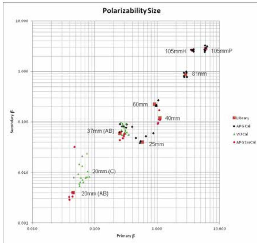
**Figure 10:** Plot of secondary vs. primary polarizability amplitude for calibration items. Points include individual results from the West Jefferson and APG Calibration grids, as well as the final library reference point used for classification of the APG grids.
