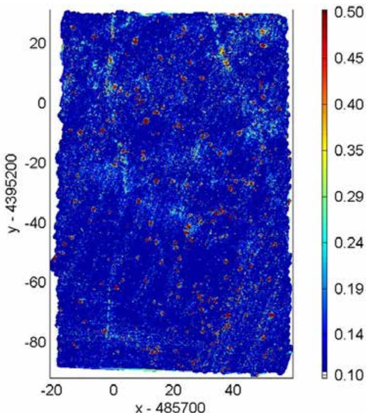
**Figure 4:** Detection map created from dynamic MPV data collected at Camp George West, CO. A detection channel of 1.4ms was used to exclude some of the fast decaying anomalies. Walking trails that passed through the survey area are evident running in a north-south orientation. Units for both horizontal and vertical axes are meters and colour scale units are mV/Amp.
