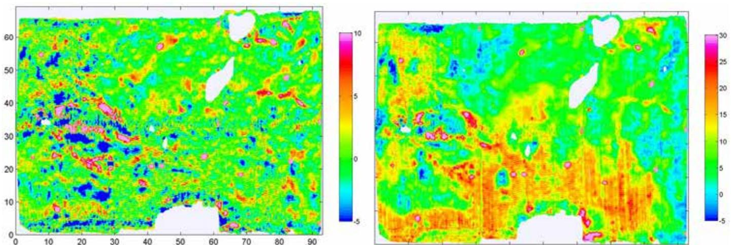
**Figure 9:** EM61 data acquired at Waikoloa TO20 Area A South. Median filtered data (on left) and the data leveled to show geology (on right). The regions of negative values in the median filtered data image are due to filtering artifacts. Units for both horizontal and vertical axes are meters and colour scale units are mV/Amp.
