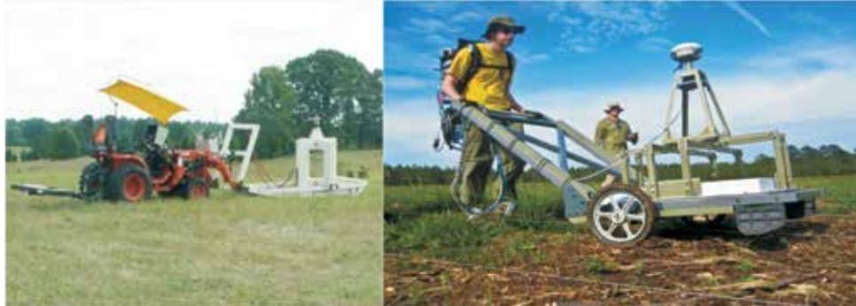
**Figure 1:** Advanced EMI sensors designed for UXO Classification. The system on the left is the MetalMapper which uses three orthogonal-axis transmitter coils and seven 3-dimensional (3D) receiver sensors called cubes. The system on the right is the TEM TADS 2x2x3D, which uses four vertical-axis transmitter coils with 4 3D receiver cubes.
