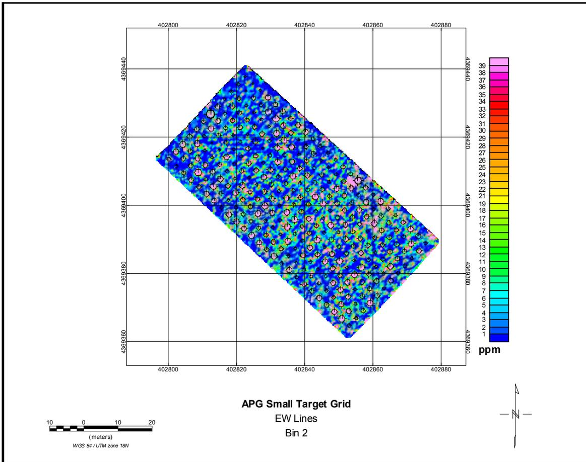
**Figure 8:** Bin2 response over the APG Small Target Grid with 20mm/37mm/40mm targets at depths to 20x diameter after removal of background response.
