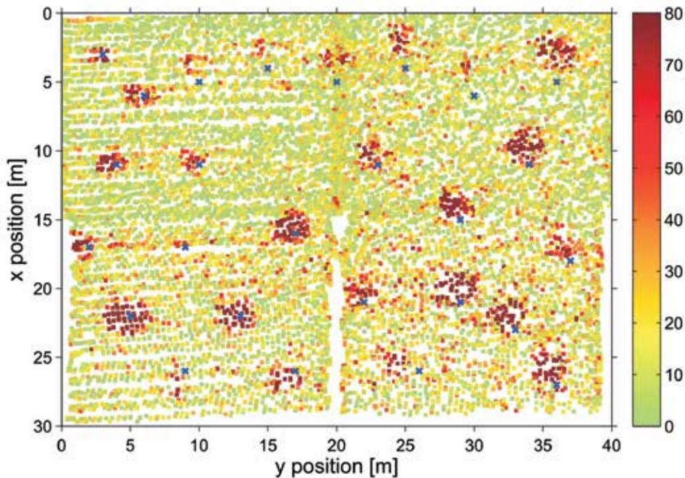
**Figure 4:** Survey results from the test area. Blue crosses indicate the positions of targets. (Data values are proportional to induced voltage output of detector.)
