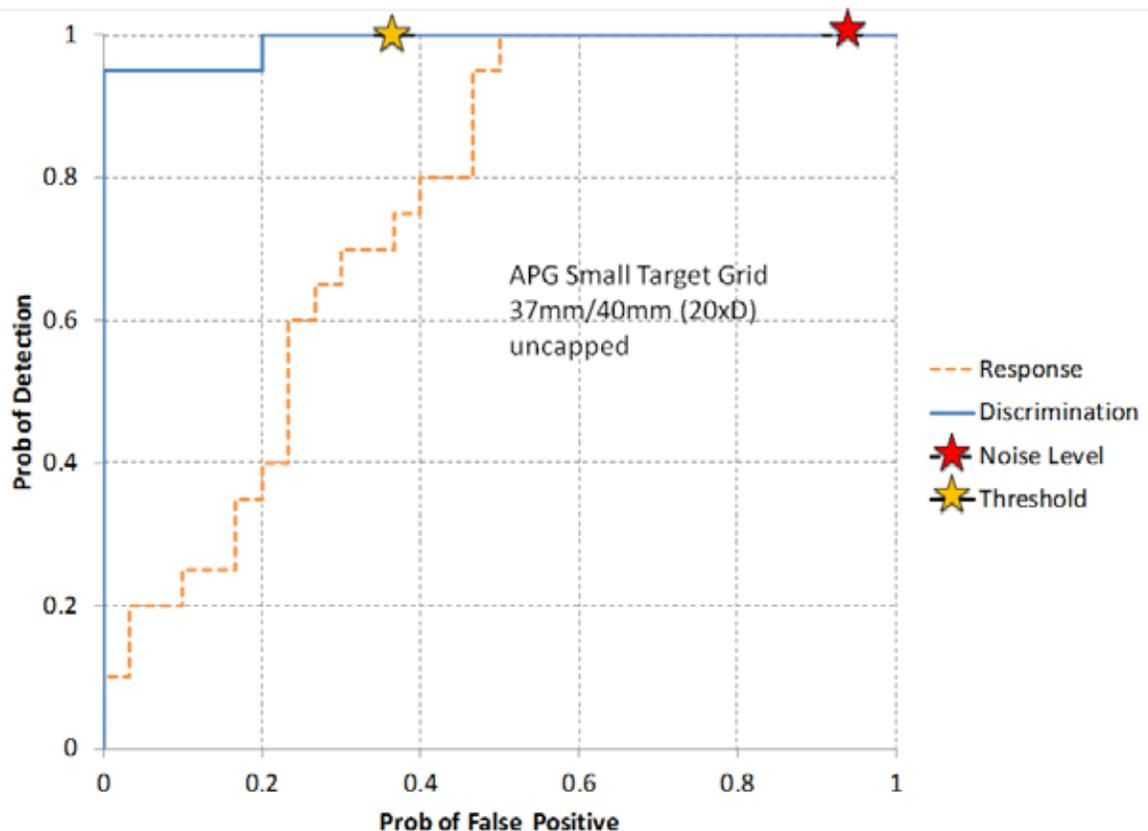
**Figure 14:** ROC curve for 37mm/40mm targets to depths of 20x diameter excluding cluttered cells.
