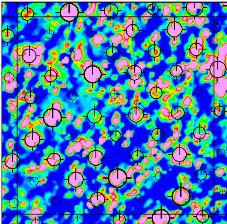
**Figure 9:** 20m x 20m extract of the Small Target Grid response in ppm (color scale is the same as Figure 8) after removal of background response to illustrate anomalous responses from seeded targets and native clutter.
