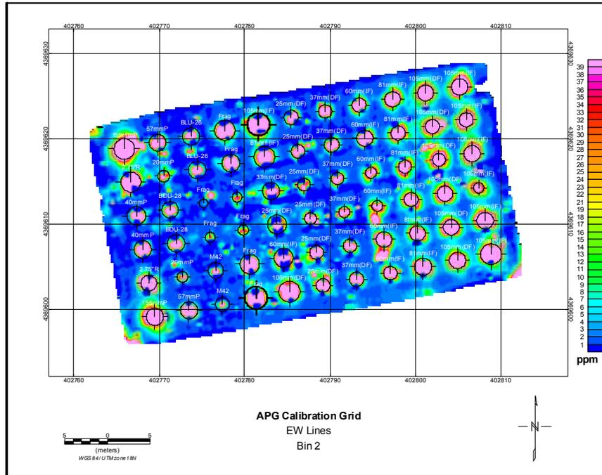
**Figure 4:** Bin2 response over the APG Calibration Grid with targets at depths to 11x diameter.
