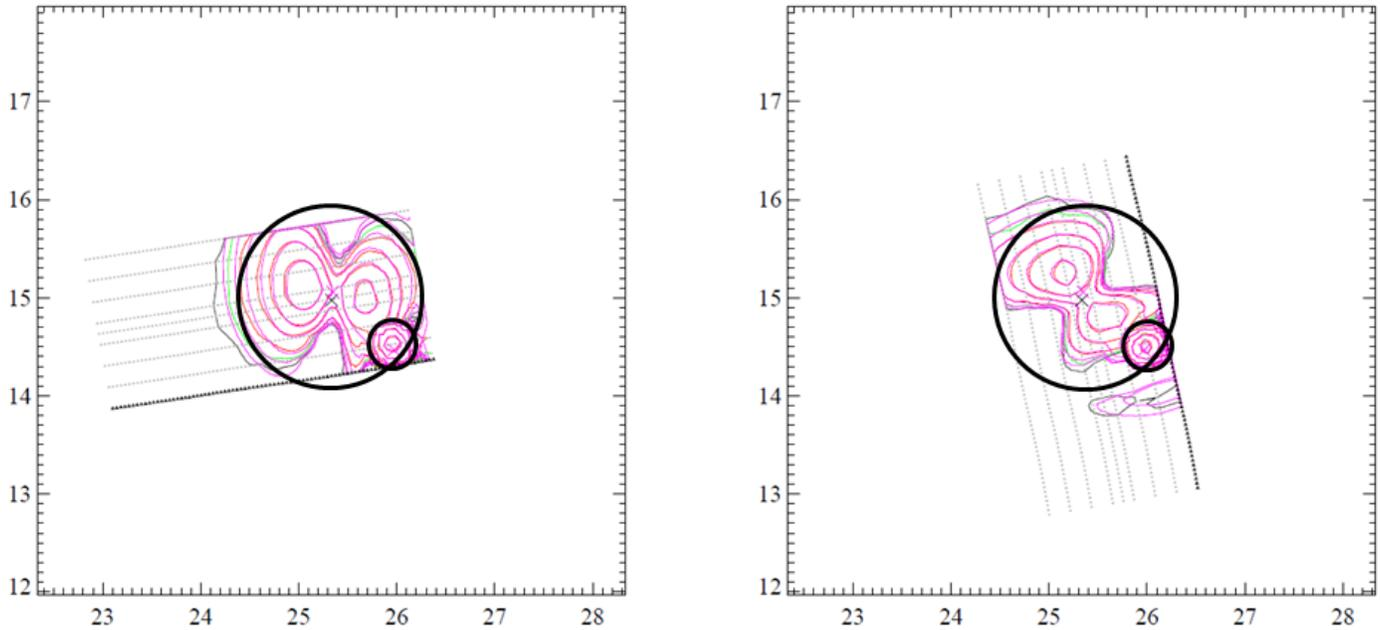
**Figure 12:** EW and NS profiles over APG Calibration Grid cell F4 showing seeded item and unintentional clutter item at 0.87m offset from the seed item. Signatures overlap but both are clearly resolved as separate items and can be inverted. Contour lines represent values in ppm.
