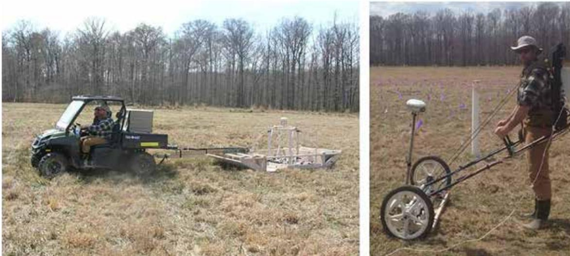
**Figure 7:** Vehicle-towed (LEFT) and man-portable (RIGHT) systems during DGM surveys at one of the DOD Standardized UXO Technology Demonstration Sites.
