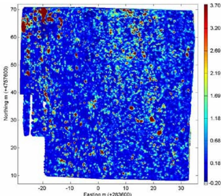
**Figure 8:** MPV detection map for New Boston AFS. The left third of the image was collected in a heavily wooded environment while the rightmost 2/3 were collected in an open field. Units for both horizontal and vertical axes are meters and colour scale units are mV/Amp.
