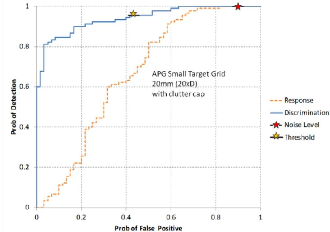
**Figure 17:** ROC curve for 20mm targets only to depths of 20x diameter with clutter cap included.
