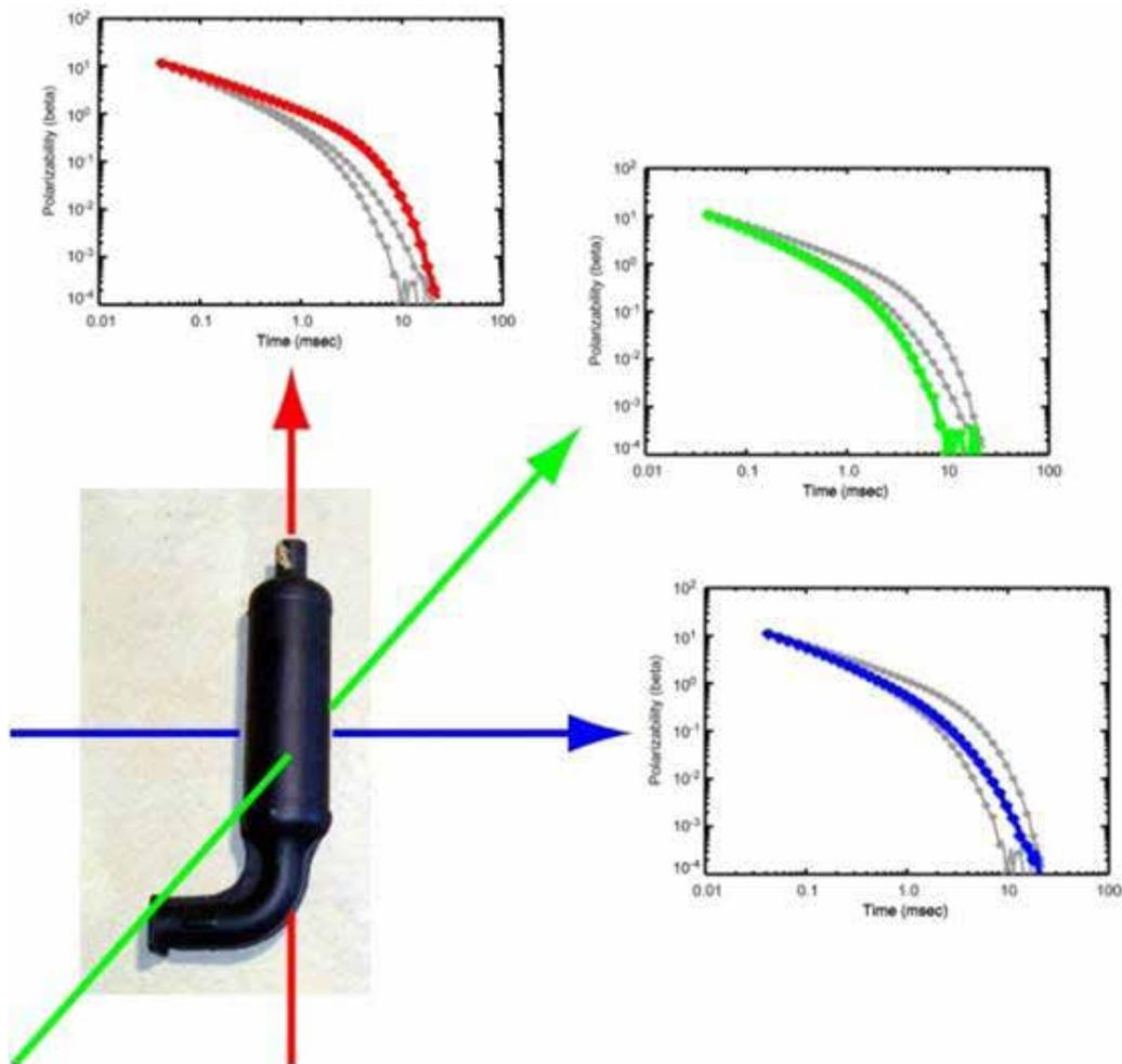
**Figure 4:** Similar to the 105mm depicted in Figure 3,  $\beta_1$  is stronger than both  $\beta_2$  and  $\beta_3$  for a muffler. However, due to the elbow,  $\beta_2$  is now stronger than  $\beta_3$ . Furthermore, due to the thinner metal, the response decays much quicker in time. (X-axis in msec and Y-axis is polarizability in beta values.)
