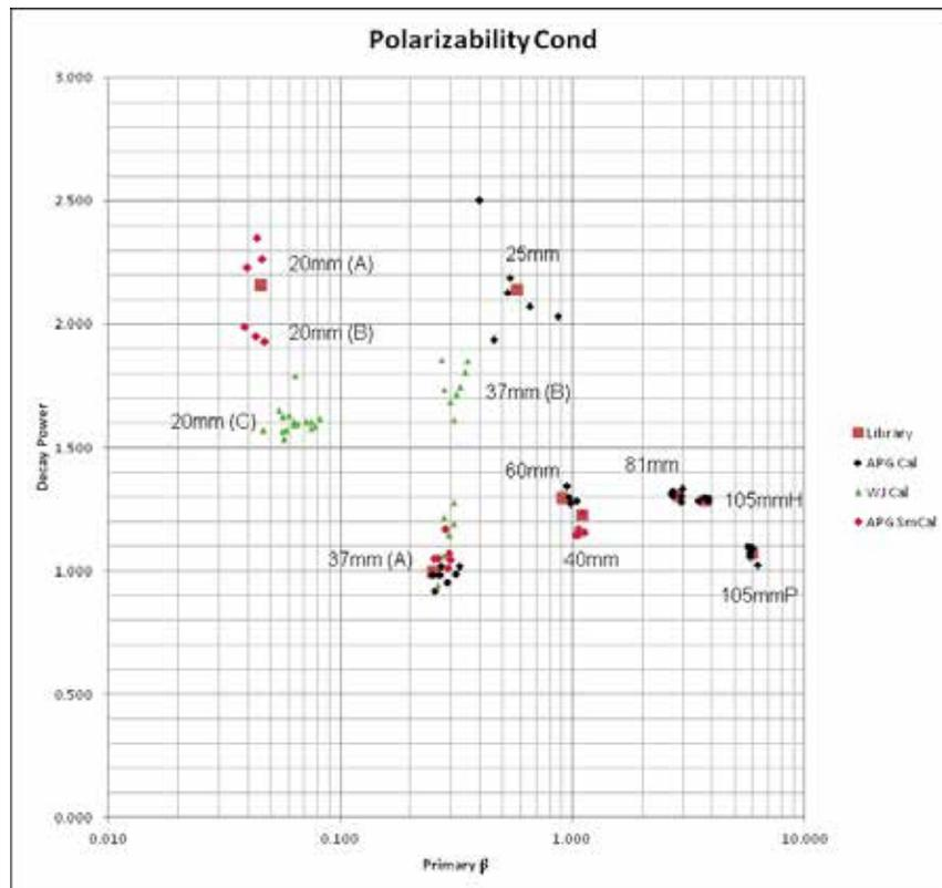
**Figure 11:** Plot of primary polarizability decay power vs. amplitude for calibration items. Points include individual results from the West Jefferson and APG Calibration grids, as well as the final library reference point used for classification of the APG grids.
