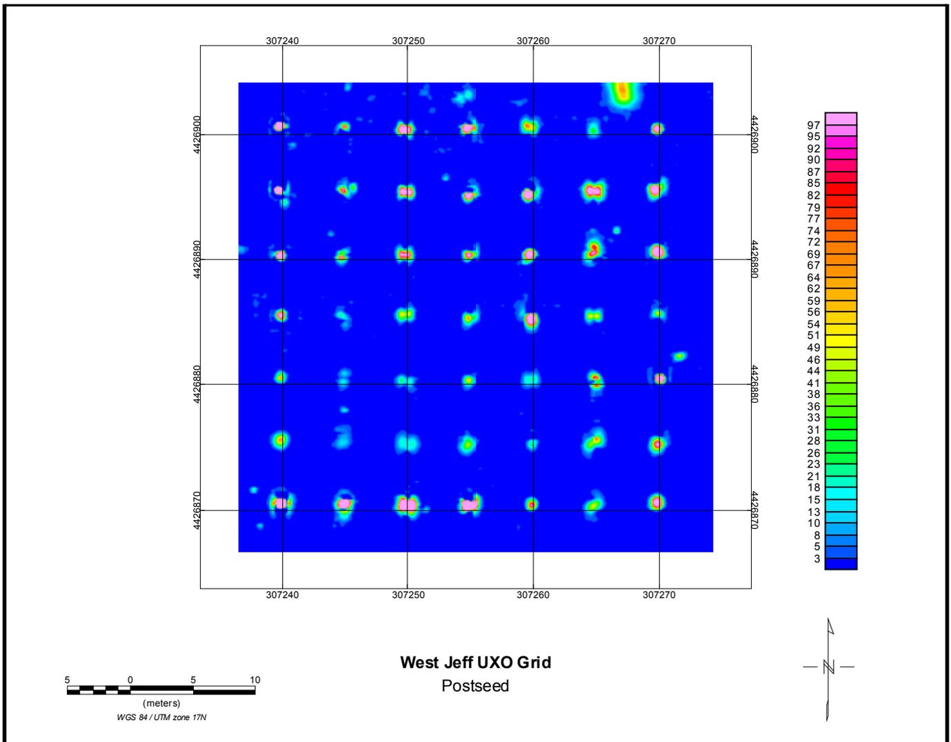
**Figure 3:** Bin2 response over the West Jefferson test grid with 20mm, 37mm, and clutter at depths to 20x diameter. Measurement units in ppm.
