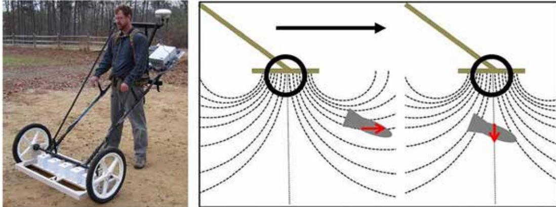
**Figure 5:** LEFT: The EMPACT man-portable array includes a single 1.0m wide by 0.5m long horizontal transmitter coil and 5 triaxial receivers. RIGHT: Because the sensor utilizes a single transmitter, effective classification is performed using a combination of multiple soundings along a transect line. As the array passes over the target, the change in the magnetic field (dashed lines) incident angle produces different angles of excitation within the target (indicated by red arrows).
