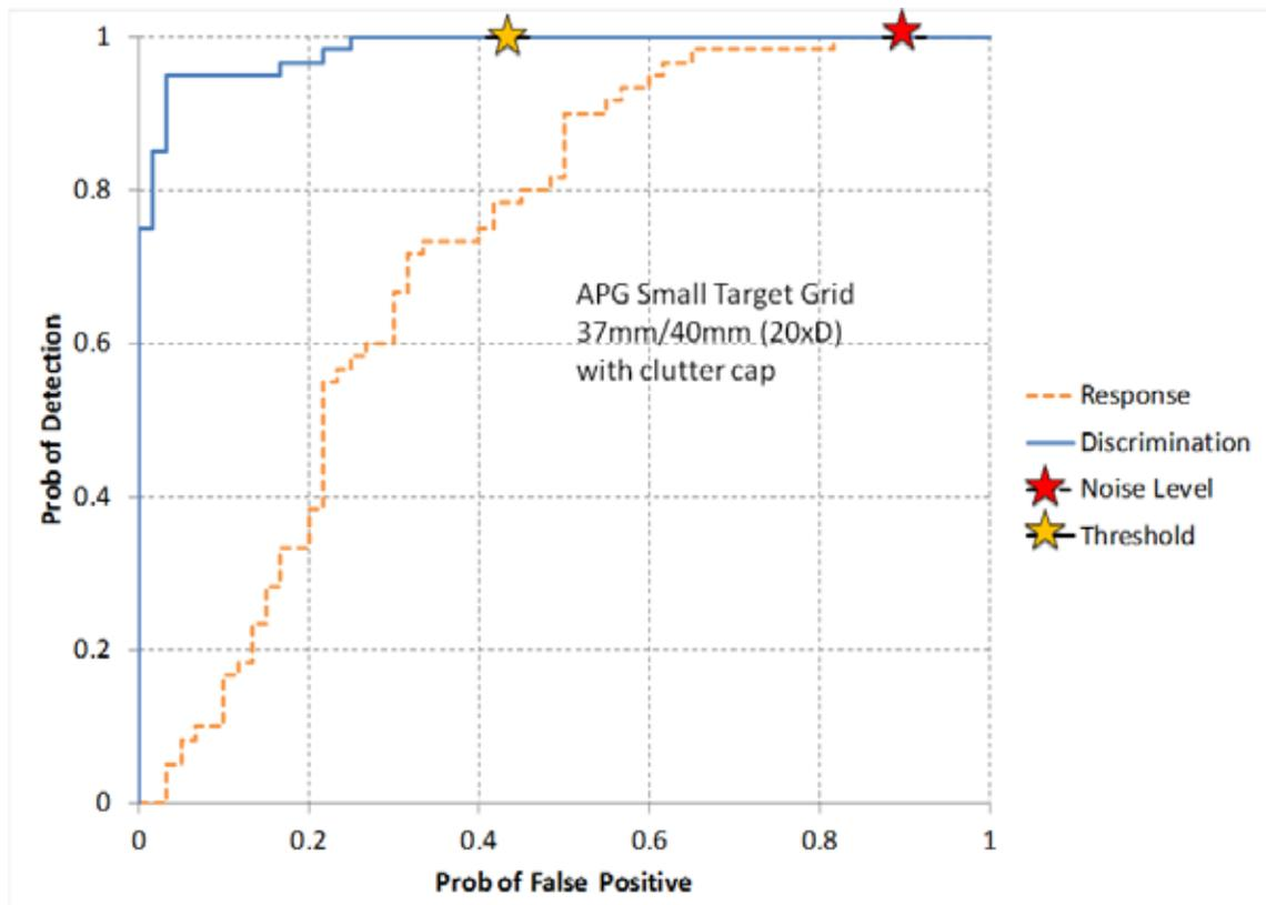
**Figure 16:** ROC curve for 37mm/40mm targets to depths of 20x diameter with clutter cap included.
