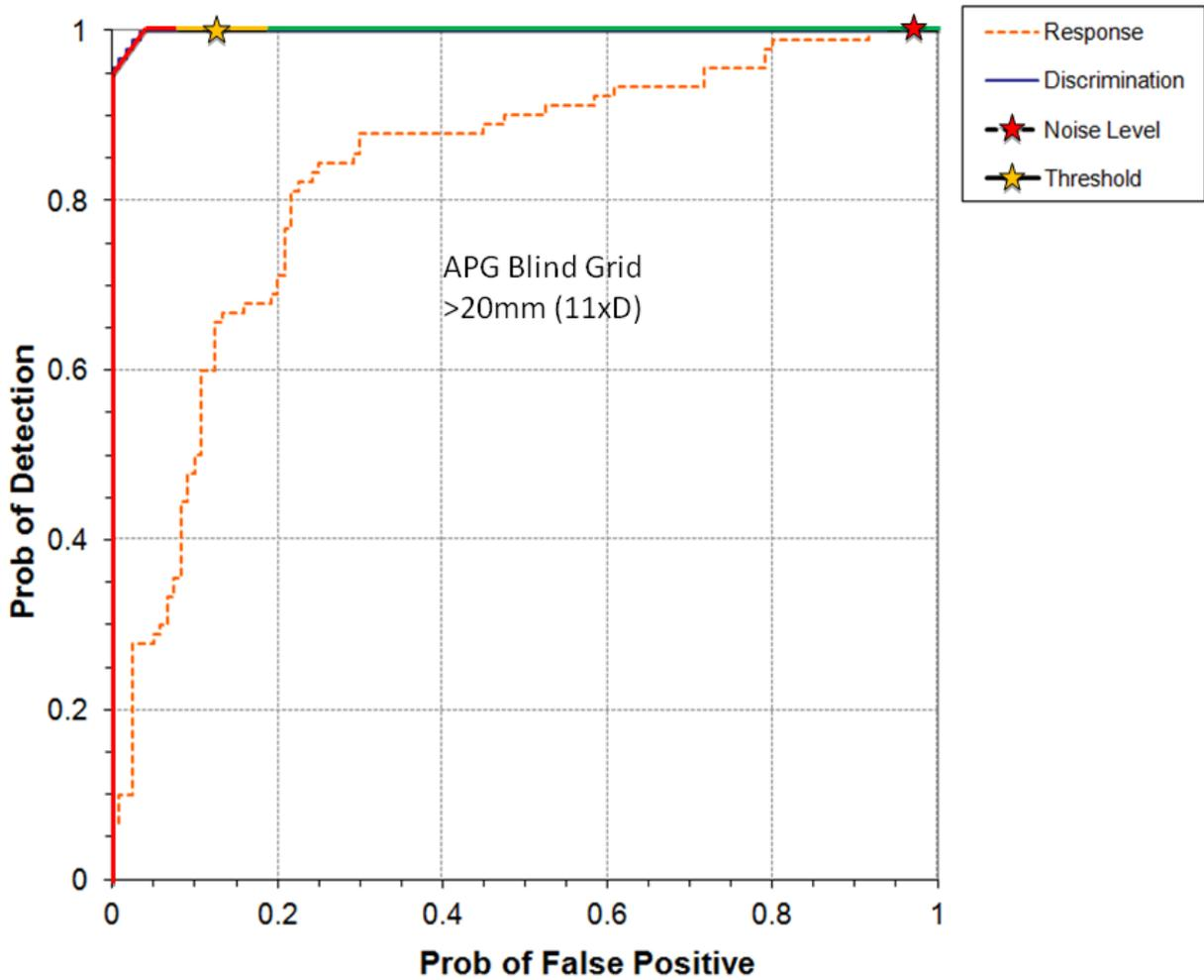
**Figure 13:** ROC curve for all targets on APG Blind Grid (>20mm, depths to 11x).
