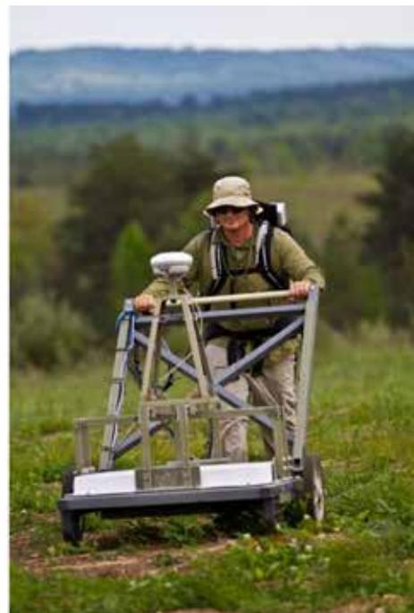
**Figure 2:** Figure 2a (left) depicts the coil configuration for the Naval Research Lab TEMTADS. Each of the boxes labeled 1-4 contain a Z-axis transmitter and a cube with three orthogonal receiver coils. Figure 2b (right) shows dynamic data collection with the TEMTADS.
