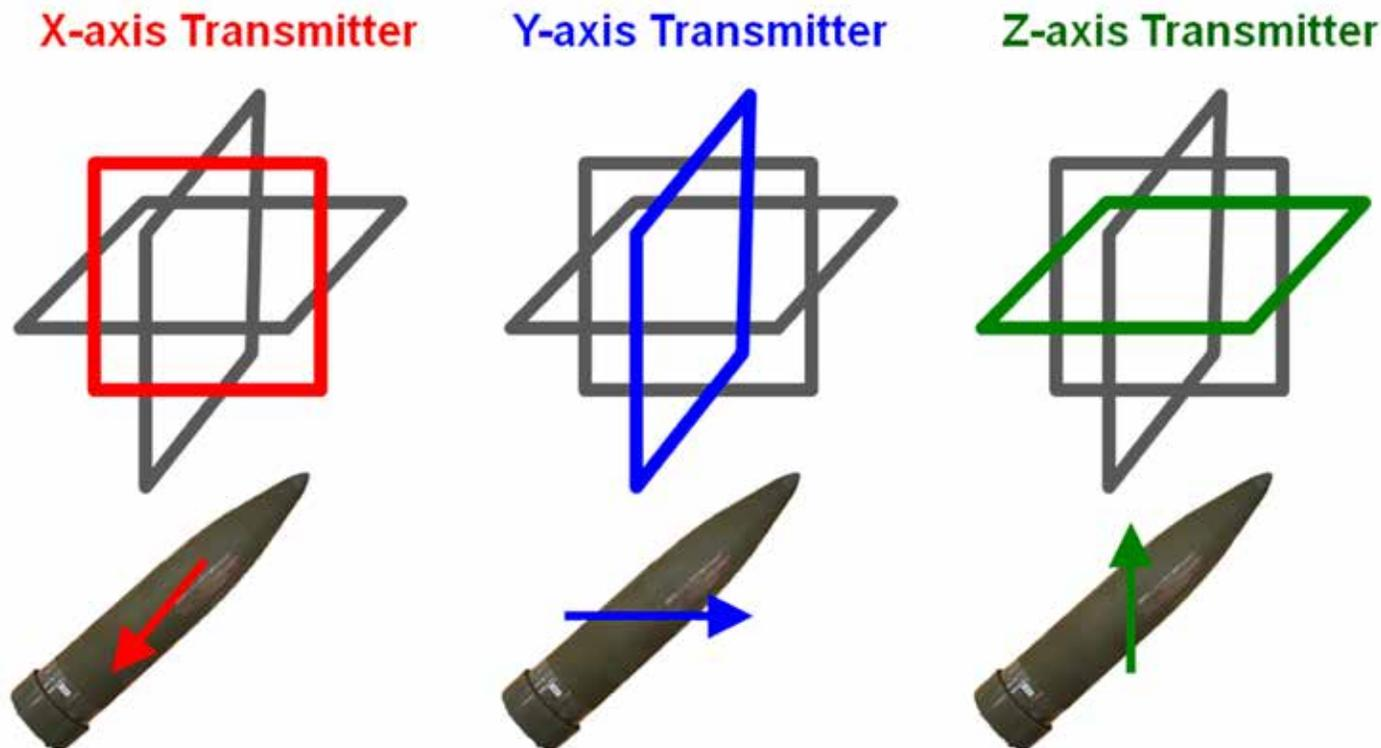
**Figure 1:** Advanced EMI sensors provide multi-axis illumination of an object by using multi-directional transmitters (TOP). Each transmitter produces a field that energizes a unique component of the object under interrogation (BOTTOM).
