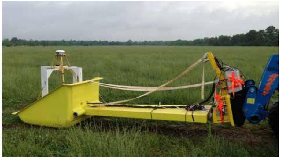
**Figure 1:** Figure 1a (left) depicts the coil configuration for the Geometrics MetalMapper. In red, blue, and green are the orthogonal transmitter coils. The cubes labeled numbers 1-7 each contain three orthogonal receiver coils. Figure 1b (right) shows a typical deployment platform for MetalMapper.
