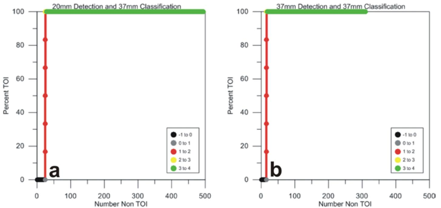
**Figure 7:** (a) ROC curve of reclassified data with the goal of detecting 20mm to a depth of 15cm and classifying 37mm or larger TOI. (b) ROC curve of reclassified data with goal of detecting and classifying 37mm to a depth of 15cm.
