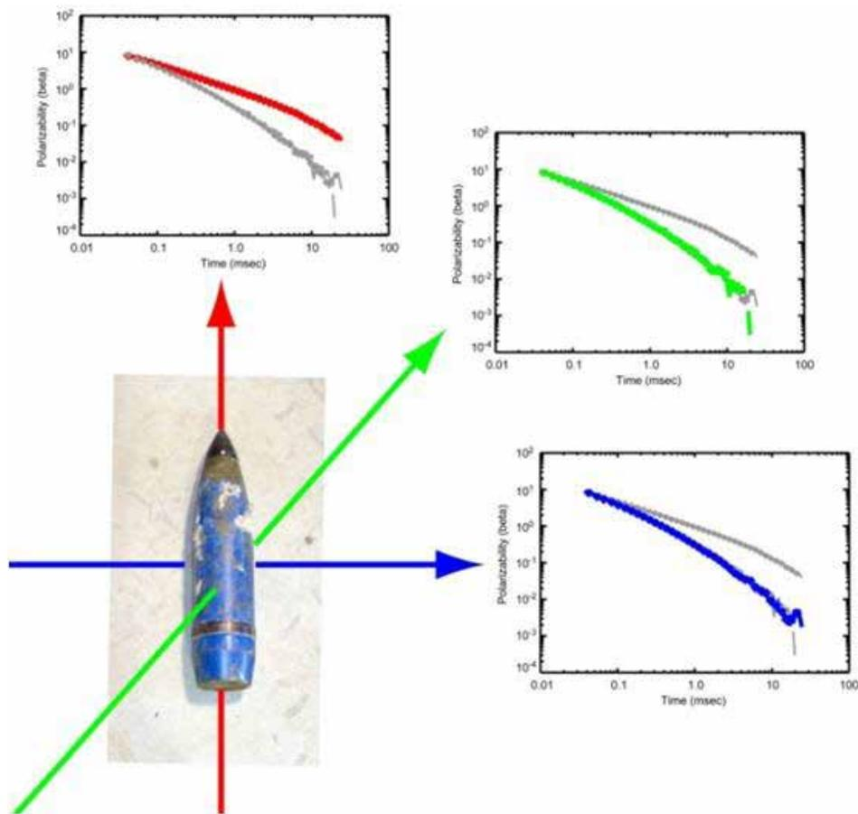
**Figure 3:** Intrinsic responses, or polarizabilities, along the principal axis directions of a 105mm. Illumination of target and receiver response from all directions allows for a fully characterized EMI signal. As expected from a cylindrical object,  $\beta_1$  has a stronger amplitude response than  $\beta_2$  and  $\beta_3$ , which are equal. (X-axis in msec and Y-axis is polarizability in beta values.)
