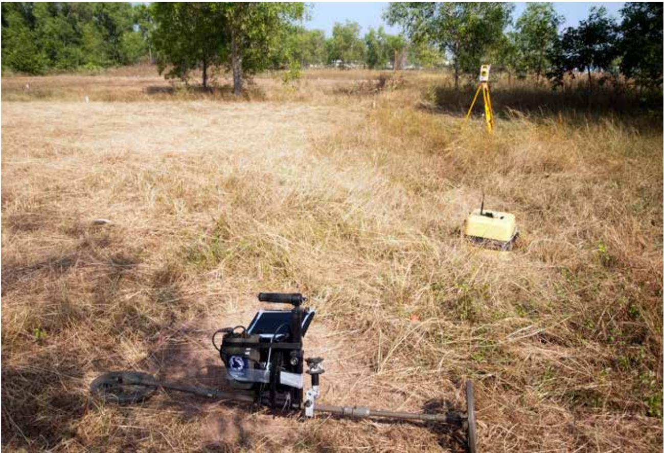
**Figure 1:** UXO detection system combining MIL-D1 DS and a total station. The sensor part also contains data acquisition computer and prism. The communication between the computer and total station is wireless using a Bluetooth transmitter.
