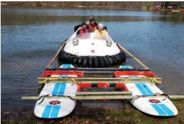
*In an early prototype developmental model Neoteric hovercraft, the TEMA system is tested and evaluated to determine the optimal pivoting and pushing system.*
