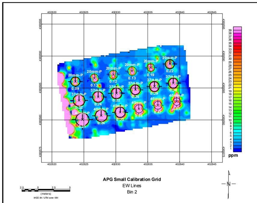
**Figure 5:** Bin2 response over the APG Small Calibration Grid with targets at depths to 11x diameter.
