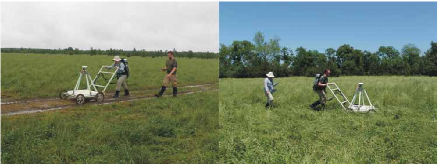
**Figure 3:** Data collection with the TEMTADS 2x2 cart at SWPG.
