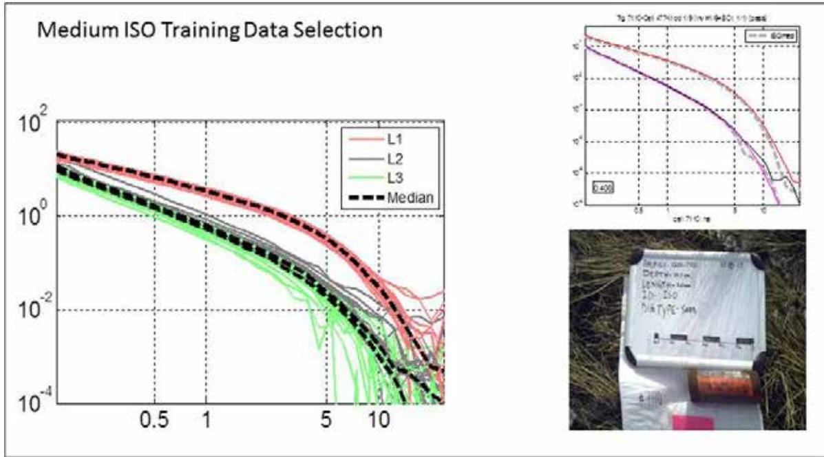
**Figure 5:** Cued data classification - Training data requests for potential medium ISOs. Plot on left shows all polarizabilities matching the reference medium ISO. The top plot on the right shows polarizabilities for a training data request (the reference library medium ISO is the dashed grey line) and the bottom right ground truth photo confirms a medium ISO. Units on the horizontal axis of polarizability plots are time in milliseconds while vertical axis units are dimensionless amplitude.
