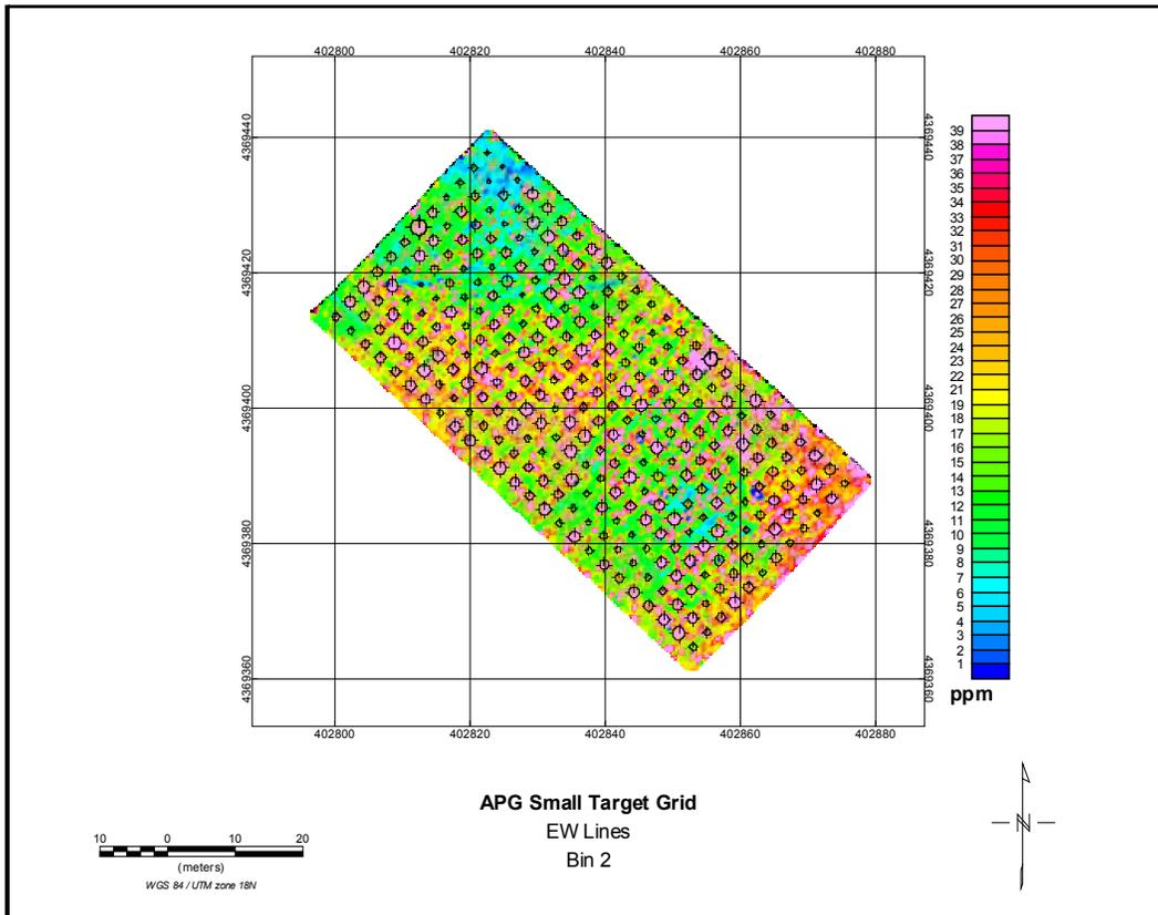
Figure 7: Bin2 response over the APG Small Target Grid with 20mm/37mm/40mm targets at depths to 20x diameter before removal of background response. Note change in background response levels from other APG sites.
