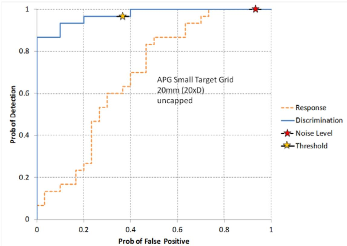
**Figure 15:** ROC curve for 20mm targets to depths of 20x diameter excluding cluttered cells.
