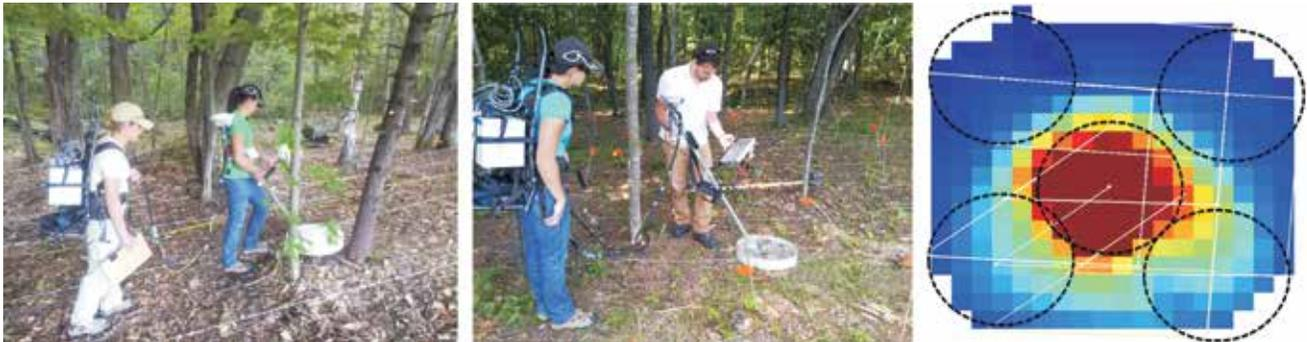
**Figure 7:** On left: Dynamic MPV surveys at New Boston AFS in a wooded area. MPV sensor is moved along short segments of well-defined lanes to build a detection map. In middle: Cued MPV surveying at New Boston AFS. On Right: Five-point static measurement pattern for MPV measurements.
