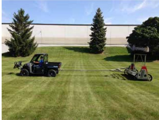
**Figure 1:** Photo of TEM-8g instrument cart and tow vehicle.
