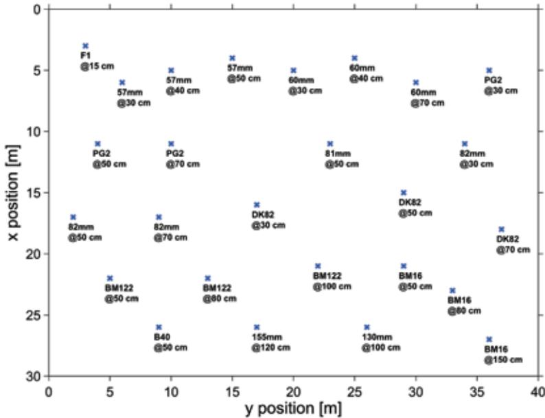
**Figure 2:** Positions, types, and burial depths of the targets planted in the test area.
