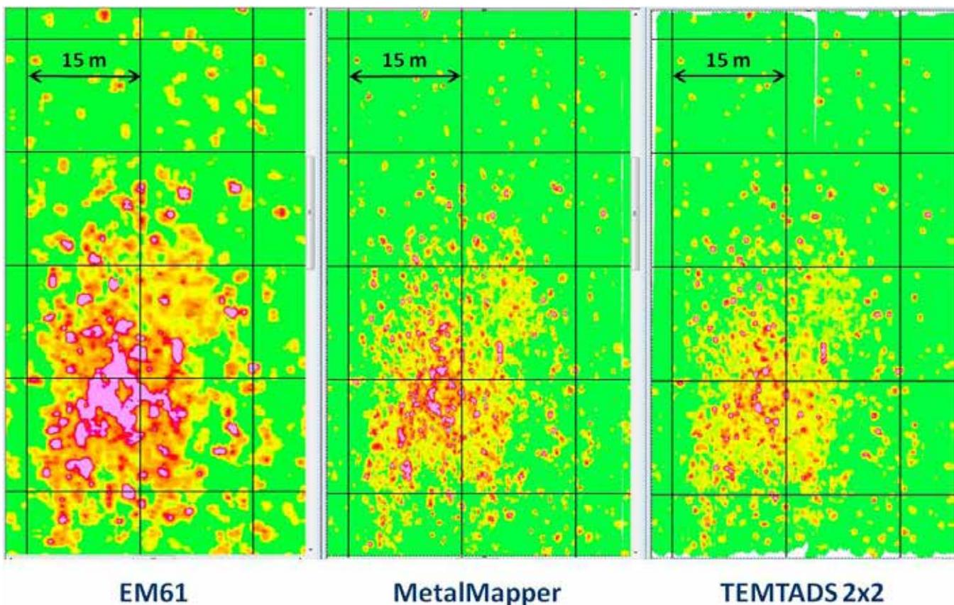
**Figure 5:** Figure 5 depicts the varying resolution capabilities of the three common instruments. Due to the greater number and smaller receiver coils, the advanced EMI sensors can better resolve individual anomalies. Future work aims to utilize more components of the data than simple amplitude thresholds which could result in the ability to better resolve, and potentially classify, targets. (EM61 measurement units are mV and MetalMapper and TEMADS 2x2 measurement units are mV/amp.)
