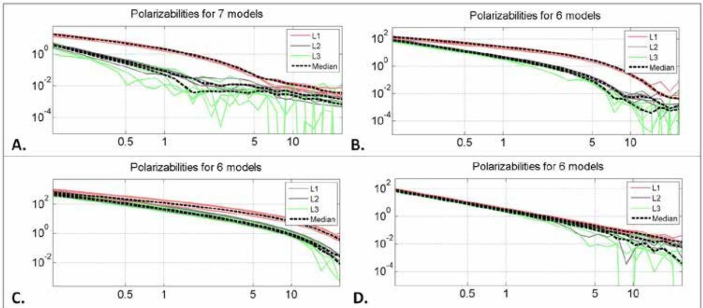
**Figure 11:** MPV3D recovered polarizabilities for 4 IVS items. A. Small ISO at 11 cm depth, B. Medium ISO at 12 cm, C: Large ISO at 16 cm, D: Sphere at 19 cm. These MPV3D derived polarizabilities were an excellent match to the IVS polarizabilities derived from MPV five-point measurements. Units on the horizontal axis of polarizability plots are time in milliseconds while vertical axis units are dimensionless amplitude.
